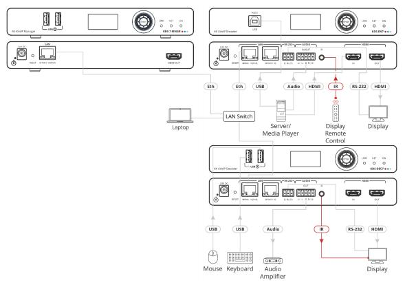
Figure 15: IR Signal Routing
