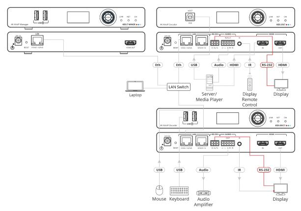
Figure 19: RS-232 Signal Routing
